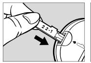
**5** Remove Test Strip from packet. Holding the round end, insert the strip fully into the Meter.
